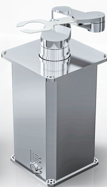
伯努利单臂机械臂 Bernoulli single-arm robot
