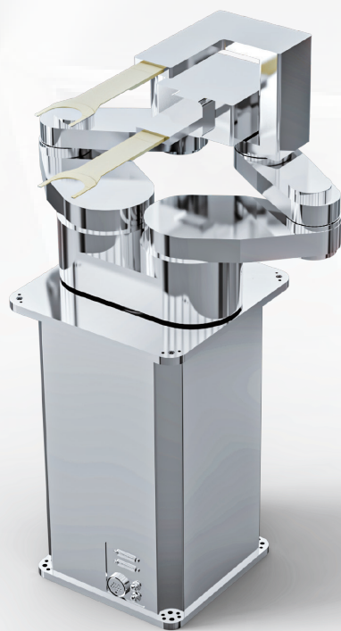
真空吸附式双臂FLIP ROBOT Vacuum adsorbing double arm FLIP ROBOT
